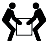
Figure 1. Lifting the centrifuge at both sides.
